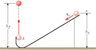
**E4**. The skateboarder in the drawing below starts down the left side of the ramp with an initial speed of 5.40-m/s. If non-conservative forces, such as kinetic friction and air resistance, are negligible, what would be the height h of the highest point reached by the skateboarder on the right side of the ramp? (**1.49-m**)
