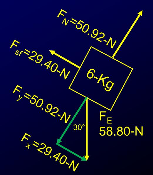
Component vectors must be put back together at the end.
