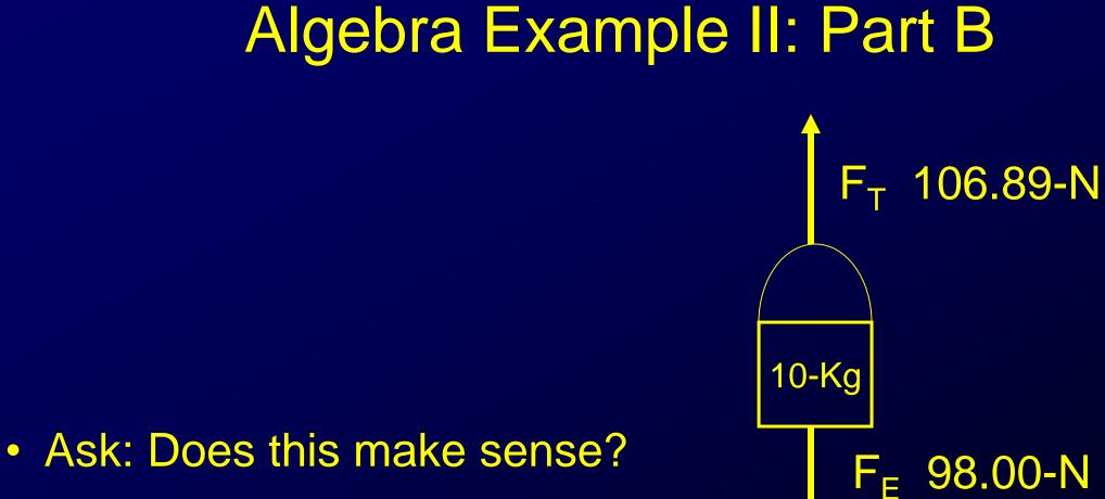
This is an example of an unbalanced force combined with no Normal force.
