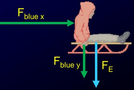
Common reaction pairs: -Push/Pull  $\leftrightarrow$  Friction: Always parallel to surface and opposite direction of travel. -Into Surface  $\leftrightarrow$  Normal Force: Always perpendicular and out of surface.
